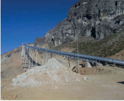
Gold Mine - Peru Overland Conveyor of 1,5 km 1 horizontal curve with radius of 800 m
