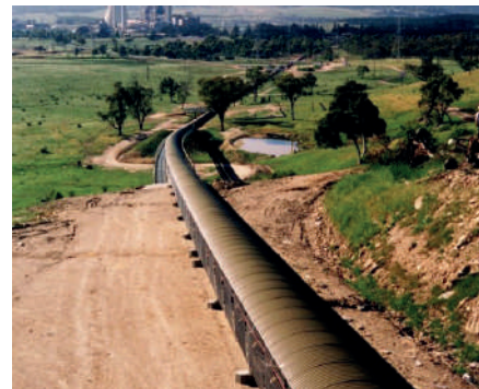
Coal mine - Australia Overland Conveyor of 4 km Bidirectional conveyor with raw coal on carry side and washed coal on return side
