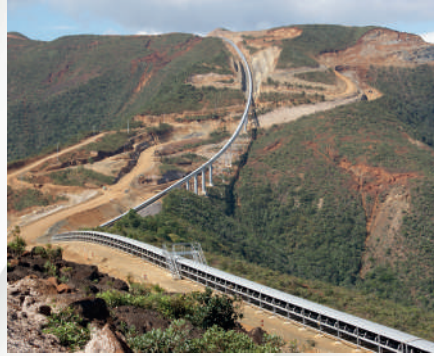
Nickel Mine - New Caledonia Overland Conveyor system of 11 km Generation of Power during operation ( 700 kW )
